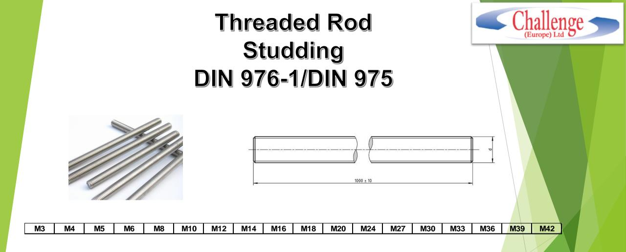
For use as tie rods or for suspending ceilings, trunking, ducting etc. Long connector nuts available. Also known as all thread or threaded bar. They are Available in 1, 2 or 3 metre lengths. Material: Zinc plated steel, also high tensile steel, brass and stainless steel.
